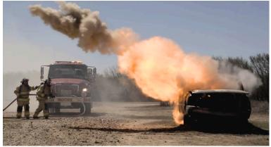
As Electric Vehicles (EV) gain popularity, firefighters more frequently face the risks associated with Thermal Runaway. The failure of Lithium-ion creating a chain reaction of uncontrollable battery temperature and internal pressure increasing inside the cell or pack, ultimately leading to gas leakage, fire, and explosion.
